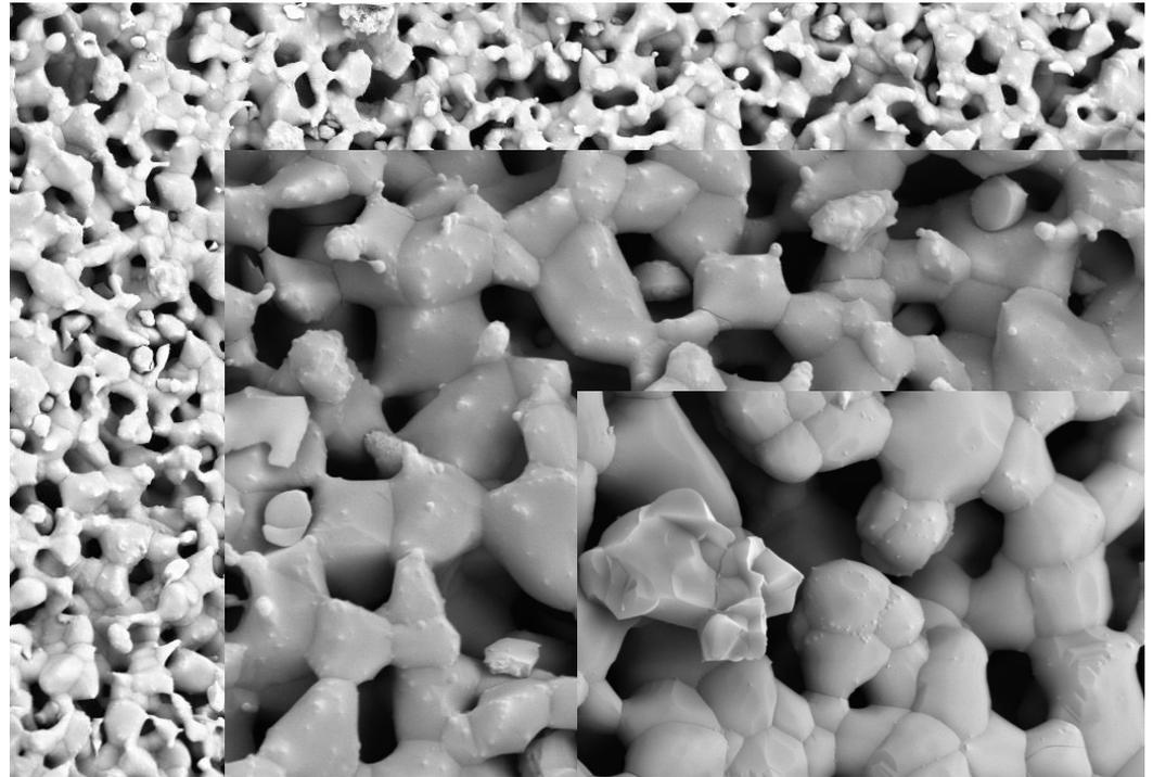
SEM images showing the microporous structure of Synergoss® White granules
